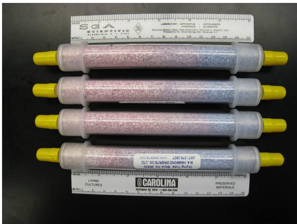
Figure 15. Condition of the four Drierite tubes from Test 4, after 5 hours of continuous operation at Lab RH of 45.1%. Average consumption was estimated to be about 70% of 32 g.
