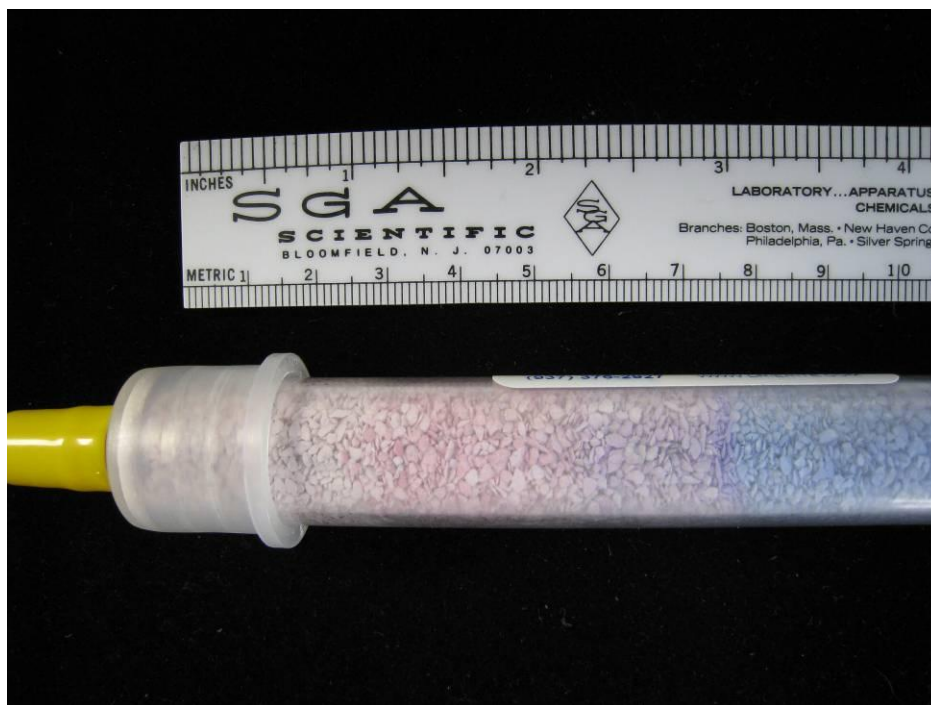
Figure 16. Zones of drying in a 15-cm Drierite 26930 tube after hours of continuous use. Five zones are observed from right: 1. 50% unused, 2. fine dark purple primary active front, 3. light purple band, 4. pink band of depleted Drierite, 5. finally white, completely exhausted Drierite. With this degree of use, there was no apparent effect on Fumiscopes zeros, as all continued to operate with little drift after warm-up.
