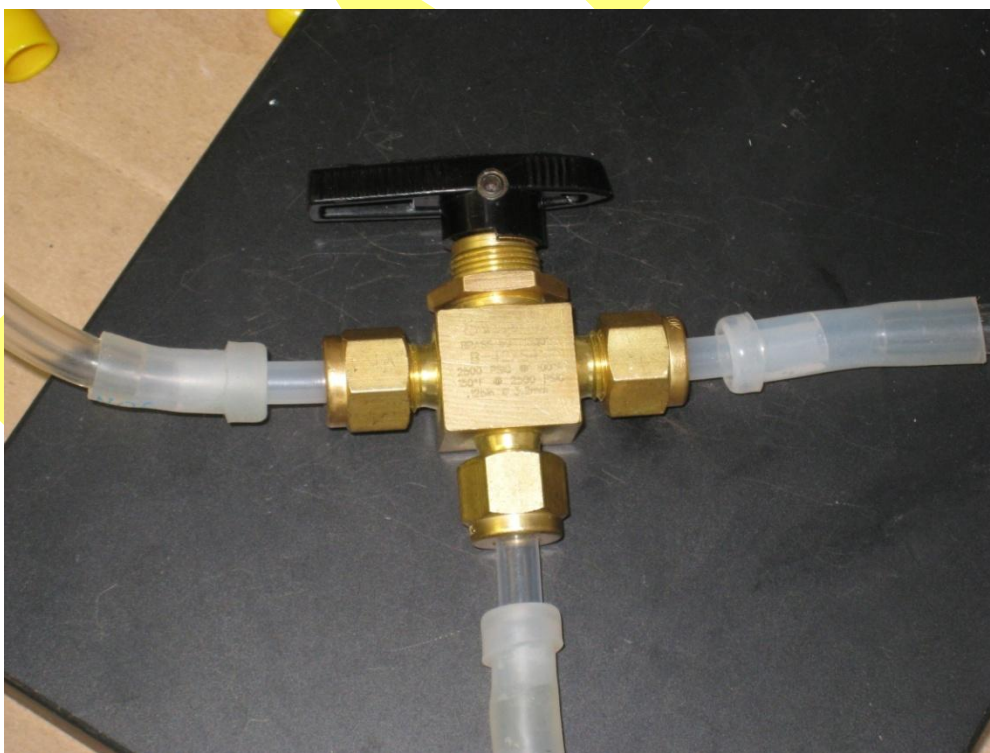
Figure 1a. Upper, Fumiscope with Swagelok B-43XS4 3-way valve to divert zero air from used Drierite to fresh Drierite tube. Lower, brass 3-way Swagelok valve with 0.25 in compression fittings. Also available with 1/8" female NPT thread and male thread brass hose barb push-on tube connections, purchased separately. In-line filter is optional.
