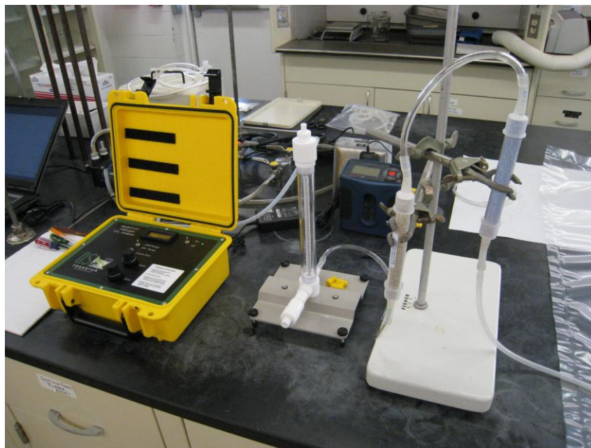
Figure 1. Set-up of the Qubit CO 2 for calibration, with (r-l) sample supply bag, Drierite tube, Ascarite (in Drierite tube), Gilmont gauge, Qubit S-157 CO 2 analyzer, and Air Cadet vacuum source.
