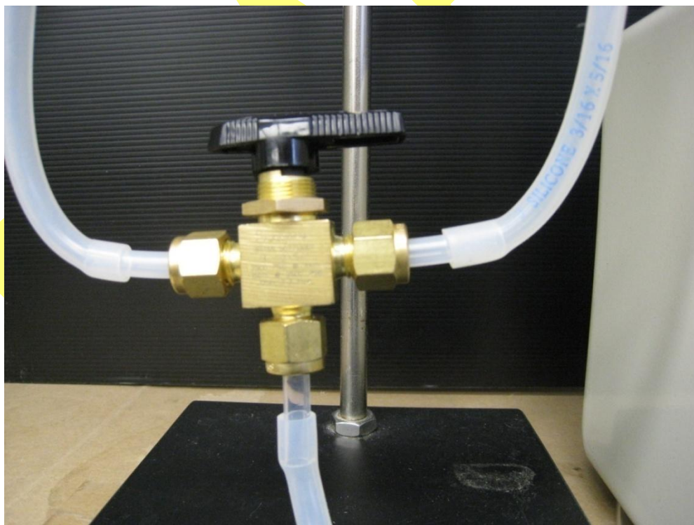
Figure 1b. Upper, Fumiscope with Swagelok B-43XS4 3-way valve to divert zero air from used Drierite to fresh Drierite tube. Lower, brass 3-way Swagelok valve with 0.25 in compression fittings. Secure connections were made with silicone 3/16 inch ID tube, which is easily cut and very flexible.
