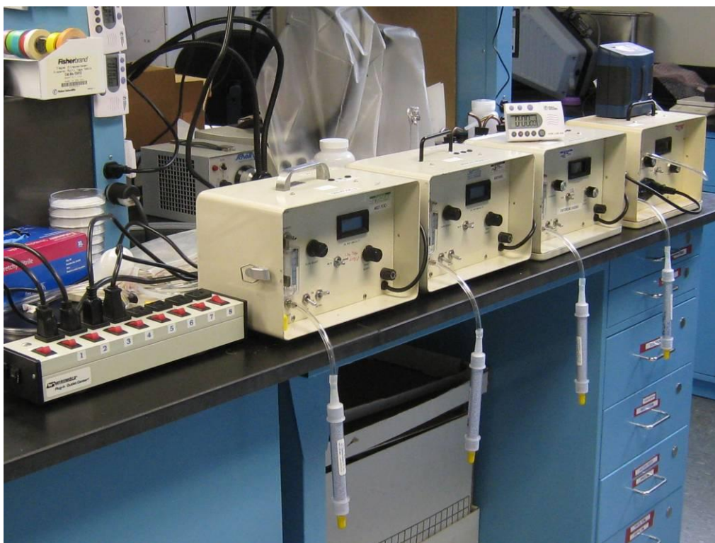
Figure 14. Lab Set-up of four Fumiscopes with attached Drierite tubes.
