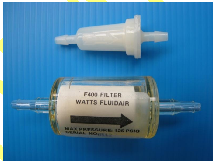
Figure 1c. Upper, experimental set-up to test effect of Ascarite on zero process by supplying alternate sources of sample air to a Fumiscoper, via a 3-way precision valve. The first supply was filtered through Drierite plus 10 g Ascarite, and the second source was filtered through only Drierite. Lower, during these tests, two types of particle filters were used. However, additional testing had shown there was no difference between filter types on zero speed or end point. Picture is approximately actual size.
