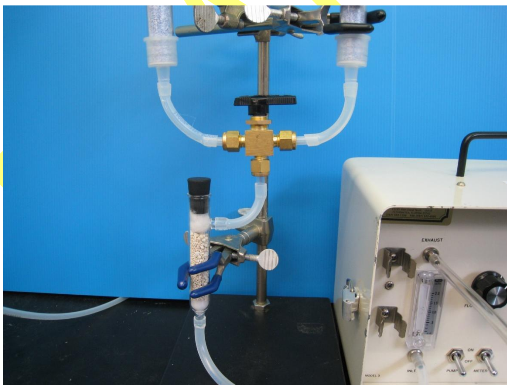
Figure 1d. Upper, Fumiscope with Swagelok B-43XS4 3-way valve to divert zero air from used Drierite to fresh Drierite tube with common Ascarite-II tube. Lower, brass 3-way Swagelok valve, with post-Drierite, shared glass tube containing 10 g of 8-10 mesh Ascarite-II.
