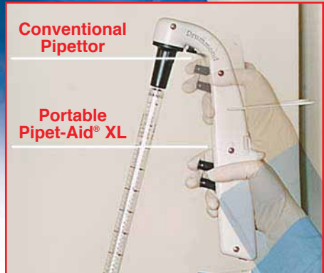
Compared to a conventional pipettor, the Portable Pipet-Aid XL lowers hand height required for the same task
